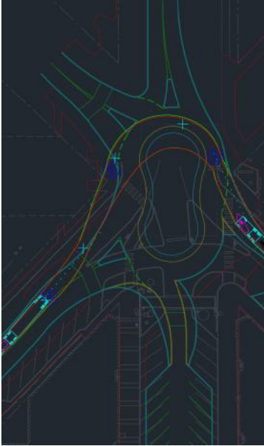
WB-50 NW PARK ST TO NE CASCADE AVE (FAILED) OPTION 1
